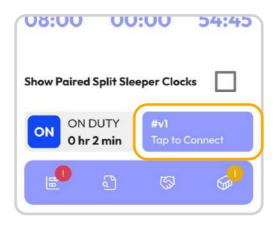
Use Tap to Connect bar to connect to your vehicle. The device will attempt to connect to selected vehicle ELD via Bluetooth. ELD bar will change from red to orange: Pairing.
